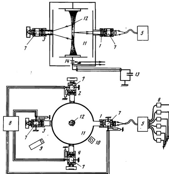
FIG. 1. Diagram of setup and arrangement of measuring apparatus: 1–4—Viewing windows, 5—MDR-2 monochromator, 6—type FEU-52 photomultipliers; 7—Kerr cells, 8—power supply for Kerr cells, 9—type ELU-FK photomultiplier with scintillator, 10—integral neutron counter, 11—vacuum chamber, 12—plasma pinch, 13—capacitor bank ( $C = 60 \mu$ F,  $U_0 = 15\text{--}40$  kV), 14—discharge gap.
