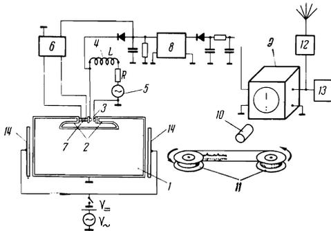
FIG. 2. Block-diagram of the measuring system: 1—the aluminum cylinder, 2—the “horns”, 3—the measuring capacitor, 4—the inductance of the transducer LC circuit, 5—pumping quartz generator, 6—servo system, 7—correcting element of the servo system (electric oven), 8—narrow-band amplifier, 9—dual-trace oscilloscope, 10—objective lens, 11—film transport mechanism, 12—receiver for standard time radio signals, 13—time marker quartz generator (quartz clock), 14—calibration system.
