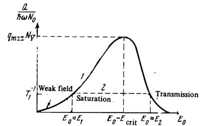
FIG. 2. Absorbed power  $Q$  as a function of the field  $E_0$  for two values of the density  $N_Y$  of the broadening particles: (1)  $N_Y \ll N_{crit}$ , (2)  $N_Y \gg N_{crit}$ .
