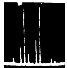
FIG. 1. Spectrum of the HF oscillations of the dynamical process established in the absence of quadratic nonlinearity ( u_0 \sim 0.3 V).
