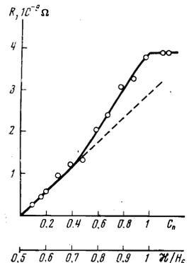
FIG. 3. Dependence of the resistance of sample 2 in the intermediate state on the concentration of the normal phase.  $T = 1.3^\circ \text{K}$ ,  $J \leq 10$  A. The dashed line is an extrapolation of the initial section of the experimental curve.
