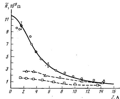
FIG. 6. Measured values of  $R$  of sample 2,  $T = 1.3^\circ\text{K}$ ,  $J_m = 15\text{ A}$ ,  $\lambda = 1.36\text{ mm}$ ;  $\circ$ — $C_N = 0.2$ ;  $\triangle$ — $C_N = 0.5$ ;  $\square$ — $C_N = 0.8$ . Solid line—theoretical curve drawn through the two points marked by the double circles.
