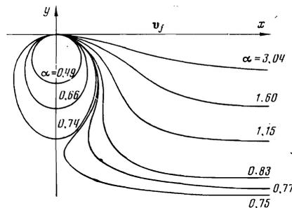
FIG. 1. Trajectory of vortex in a Gaussian potential field at  $\theta_H = \pi/2$  for various values of the "criticality" parameter  $\alpha$ .
