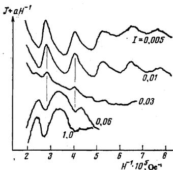
FIG. 8. Oscillations of the photocurrent at different intensities of illumination of Ge:Ga;  $T = 1.5^\circ\text{K}$ ,  $E = 3.5$  V/cm,  $H \parallel [100]$ . The two lower curves were recorded with the gain decreased by a factor of five.
