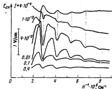
FIG. 9. Oscillations of the field  $E_{GH}$  at different illumination intensities; Ge:Ga sample,  $T = 1.63^\circ\text{K}$ ,  $H \parallel [100]$ .
