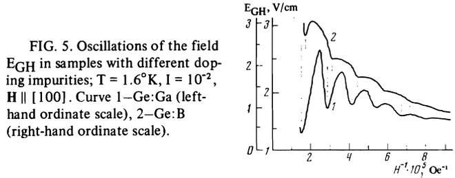
FIG. 5. Oscillations of the field  $E_{GH}$  in samples with different doping impurities;  $T = 1.6^\circ\text{K}$ ,  $I = 10^{-2}$ ,  $H \parallel [100]$ . Curve 1—Ge:Ga (left-hand ordinate scale), 2—Ge:B (right-hand ordinate scale).
