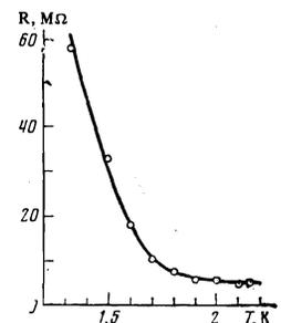
FIG. 2. Temperature dependence of the magnetoresistance. Sample G1,  $H = 21$  kOe, relative intensity  $I = \nu/\nu_{\max} = 4 \times 10^{-2}$ ,  $E \approx 1$  V/cm,  $H \parallel [100]$ .
