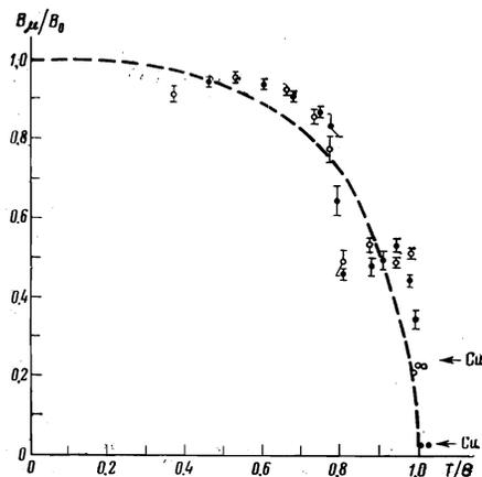
FIG. 2. The ratio  $B_{\mu}/B_0$  as a function of temperature for  $B_0 = 1760$  G. The smooth curve is the Brillouin function for the ratios  $M/M_{\text{sat}}$ .  $\Theta = 289$  K is the Curie temperature for gadolinium. The remaining designations are the same as in Fig. 1.
