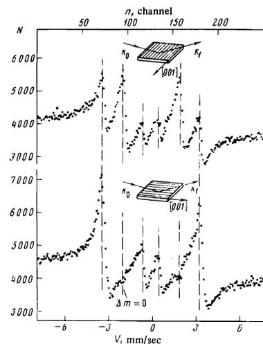
FIG. 3. Mössbauer spectra for the Bragg reflection of  $14.4\text{-keV}$  radiation from the  $(110)$  plane of an  $\text{Fe}^{57}$  crystal for two different azimuthal positions of the crystal.
