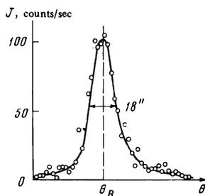
FIG. 2. Curve of the Laue reflection of  $\text{MoK}_{\alpha_1}$  x-rays from the  $(1\bar{1}0)$  plane of a crystal of  $\text{Fe}^{57}$ .
