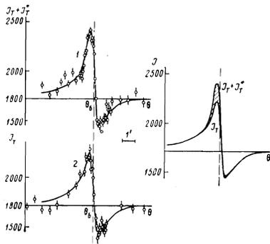
FIG. 5. The angular dependences for transmission of  $\gamma$  quanta by an  $\text{Fe}^{57}$  crystal in the vicinity of  $\theta = \theta_B$  for  $(1\bar{1}0)$  planes when the energy of the  $\gamma$  quanta is equal to the energy of the nuclear transition  $-\frac{1}{2} \rightarrow -\frac{1}{2}$ : curve 1—in the absence of the polarizer-shaper, 2—in the presence of the polarizer-shaper.
