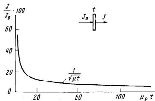
FIG. 6. Dependence of the transmission of Mössbauer radiation through a resonant absorber on the thickness of the absorber.
