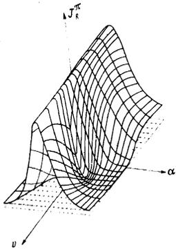
FIG. 9. Theoretical surface for Laue reflection of the  $\pi$ -polarized component of the beam in the vicinity of the Bragg angle and near the resonance energy.
