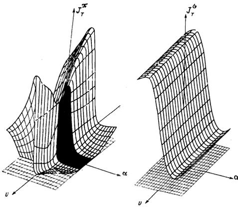
FIG. 8. Theoretical surfaces for the transmission of the  $\pi$ - and  $\sigma$ -polarized components of a  $\gamma$  beam through a crystal of  $\text{Fe}^{57}$  in the vicinity of the Bragg angle and near the resonance energy.
