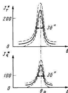
FIG. 7. Angular dependences of the transmission of the nuclearly-active component of the incident  $\gamma$  beam through an  $\text{Fe}^{57}$  crystal in the neighborhood of the Bragg angle.
