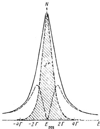
FIG. 1. Energy distribution of the  $\gamma$  quanta: solid line—in the radiation flux emitted by the source; dashed line—in the flux passing through the resonant filter; the shaded portion indicates the distribution of the quanta absorbed by the filter;  $\Gamma$  denotes the natural linewidth.
