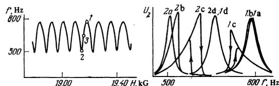
FIG. 1. Resonance frequency of the sample vs the magnetic field (single curve) and the resonance curves of the first number of the resonance of helicons at fixed magnetic field at points 1 and 2 at different values of the exciting current: a— $I=0.3$  mA, b— $I=3.0$  mA, c— $I=10$  mA, d— $I=100$  mA. When the exciting current was varied, the gain of the system was changed in the opposite direction by a corresponding amount.
