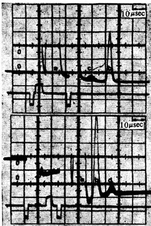
FIG. 6. Oscillograms of the echo signals in the case of the RPR pulse sequence: a) parametric-echo signal,  $t = 2t_2$ ; b) FM-echo signal,  $t = 2t_3$ ; c) secondary-echo signal,  $t = t_3 + (t_3 - 2t_2)$ ; d) secondary-echo signal,  $t = t_3 - 2(t_3 - 2t_2)$ .
