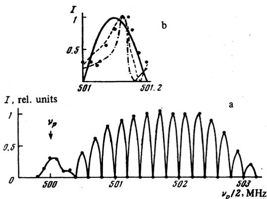
FIG. 10. Dependence of the amplitude of the parametric-echo signal on  $\nu_p/2$  for RF-field intensities  $\eta_1 h_1 = 0.1$  Oe (a) and 0.4 Oe (b) under the conditions of single-pulse formation. The dashed curve depicts the shape of the function  $A(\nu_i)$  for  $\eta_1 h_1 = 0.4$  Oe,  $\tau_r = 5$   $\mu$ sec; the dot-dash curve, the shape of the function  $A(\nu_i)$  for  $\eta_1 h_1 = 0.6$  Oe,  $\tau_r = 5$   $\mu$ sec.
