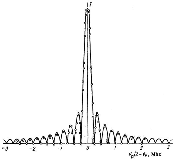
FIG. 4. Dependence of the amplitude of the parametric-echo signal on  $\nu_r - \nu_p/2$ : O)  $\tau_r = 4 \mu\text{sec}$ ,  $\tau_p = 10 \mu\text{sec}$ , and  $\nu_r$  is varied; X)  $\tau_r = 10 \mu\text{sec}$ ,  $\tau_p = 2 \mu\text{sec}$ ,  $\nu_p$  is varied; the continuous curve is the theoretical curve—the Fourier transform of a rectangular pulse of duration  $4 \mu\text{sec}$ .
