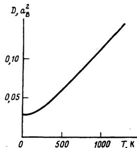
FIG. 2. Temperature dependence of the exponential coefficient of the Debye-Waller factor.
