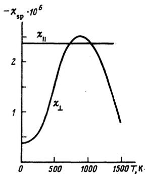
FIG. 1. Dependence of the components of the tensor of the specific magnetic susceptibility of beryllium on the temperature (in cgs specific units).
