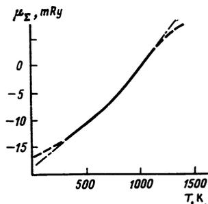
FIG. 5. Local position of the level of the chemical potential  $\mu_x$  vs. temperature. Solid curve—result of self-consistent calculation. The dashed sections of the curve correspond to  $k_E = 0.438$  (a.u.)<sup>-1</sup>, and the dash-dot ones to  $k_E = 0.4$  (a.u.)<sup>-1</sup>.
