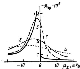
FIG. 4. Dependence of the component  $\chi_{\perp}$  of the orbital susceptibility of beryllium on the chemical-potential level at temperatures 4.2 (1), 300 (2), 900 (3), and 1500 K (4).
