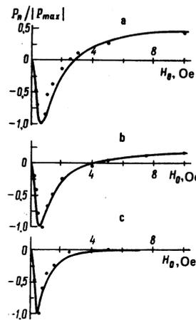
FIG. 4. Dependence of the degree of the optical polarization on  $H_0$  for: a) Si:P:Au with  $N(\text{P}) \approx 10^{16} \text{ cm}^{-3}$ ; b) Si:P:Au with  $N(\text{P}) \approx 5 \times 10^{15} \text{ cm}^{-3}$ ; c) Si:P:Au with  $N(\text{P}) \approx 10^{15} \text{ cm}^{-3}$ . The gold concentration in all three samples was  $N(\text{Au}) \approx 3 \times 10^{16} \text{ cm}^{-3}$ . The continuous curves are the calculated dependences.
