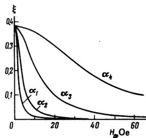
FIG. 1. Dependence of  $\xi$  on the magnetic field  $H_0$ . The values of  $\alpha_1$ ,  $\alpha_2$ ,  $\alpha_3$ , and  $\alpha_4$  are associated with  $\tau_S = 10^{-7}$ ,  $5 \times 10^{-8}$ ,  $2 \times 10^{-8}$ , and  $10^{-8}$  sec, respectively.
