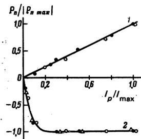
FIG. 5. Dependences of the degree of the optical polarization of the  $^{29}\text{Si}$  nuclei on the intensity of the pump radiation reaching Si:P:Au samples: 1) optical pumping in a field 10 Oe; 2) optical pumping in a field 0.7 Oe;  $\circ$ )  $N(\text{P}) \approx 10^{16} \text{ cm}^{-3}$ ;  $\bullet$ )  $N(\text{P}) \approx 5 \times 10^{15} \text{ cm}^{-3}$ ;  $\Delta$ )  $N(\text{P}) \approx 10^{15} \text{ cm}^{-3}$ .
