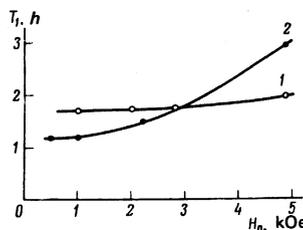
FIG. 6. Dependences of the spin-lattice relaxation time  $T_1$  of the  $^{29}\text{Si}$  nuclei on the magnetic field  $H_0$  in Si:P:Au with  $N(\text{P}) \approx 10^{16} \text{ cm}^{-3}$  (curve 1) and  $N(\text{P}) \approx 5 \times 10^{15} \text{ cm}^{-3}$  (curve 2).
