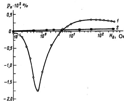
FIG. 3. Dependence of the degree of polarization  $P_n$  of the  $^{29}\text{Si}$  nuclei on the magnetic field  $H_0$  obtained for Si:P:Au (curve 1) and Si:P (curve 2) when pumped optically with circularly polarized light.
