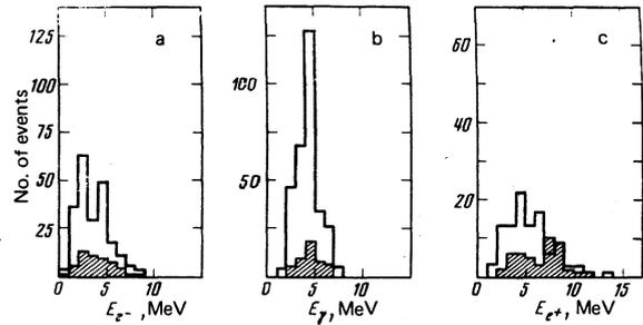
FIG. 3. Spectra of delayed particles in the propane chamber: a—electrons; b— $\gamma$  rays; c—positrons. The distributions for particles in the primary-beam region have been crosshatched.
