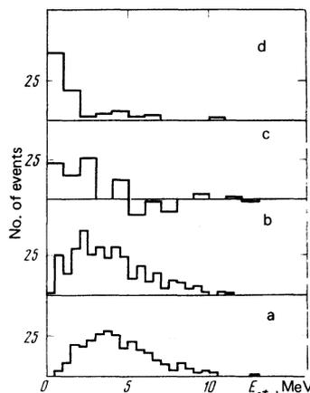
FIG. 2. Spectrum of decay electrons or positrons in the Lyudmila chamber: a—decay particles from the target along the beam; b—decay particles from the target opposite to the beam; c—the difference of spectra a and b; d—spectrum of particles in the hydrogen of the chamber.
