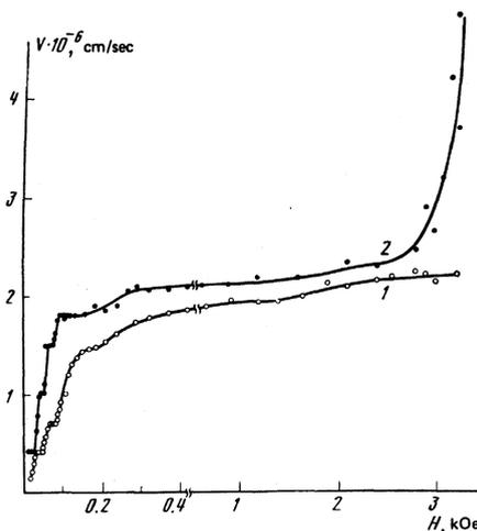
FIG. 3. Velocity of motion of single domain walls perpendicular to the specimen surface, in a chemically polished  $\text{YFeO}_3$  plate. 1) 293 K; 2) 100 K.
