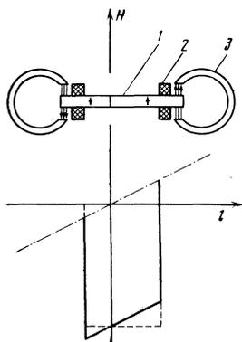
FIG. 1. Magnetic-field distribution in the specimen during domain-wall motion. 1)  $\text{YFeO}_3$  plate; 2) coils producing a pulsed magnetic field (dotted); 3) magnets producing a gradient field (dash-dotted); field acting on the specimen (solid curve).
