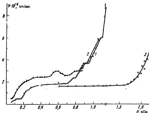
FIG. 2. Velocity of motion of single domain walls in an optically polished  $\text{YFeO}_3$  plate in a pulsed magnetic field. 1) 293 K; 2) 100 K; wall of intermediate type, perpendicular to the specimen surface; at temperature 293 K, the maximum velocity was  $2 \cdot 10^7$  cm/sec. Curve 3, 293 K; wall of Bloch type, oblique to the specimen surface.
