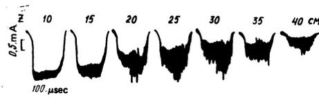
FIG. 1. Oscillograms of the beam current density,  $p = 6.7 \times 10^{-6}$  Torr.
