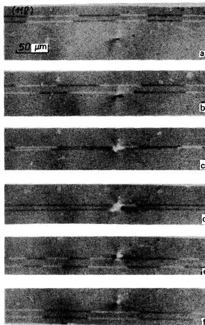
FIG. 6. Form, in linearly polarized light, of a 180-degree DB, oscillating under the action of a pulsed magnetic field of constant amplitude, under conditions such that its equilibrium position is located at various distances from an edge dislocation perpendicular to the plane of the figure, at the center of the double-refraction rosette.
