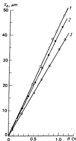
FIG. 1. Variation of the amplitude  $x_0$  of oscillation of a DB with the value of a pulsed magnetic field  $H$ , measured for various repetition frequencies of the pulse: 1, quasistatic conditions; 2,  $\nu = 2$  kHz; 3,  $\nu = 20$  kHz.
