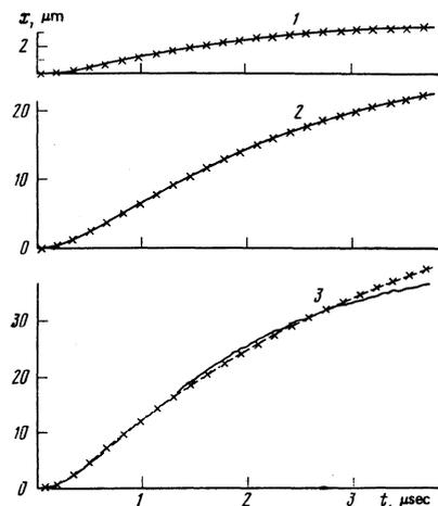
FIG. 2. Experimentally measured (solid lines) and calculated [on the basis of solution of equation (2); dotted with crosses] displacement  $x$  of a DB as a function of the time  $t$  of action of a magnetic field pulse: 1,  $H = 0.1$  Oe; 2,  $H = 0.8$  Oe; 3,  $H = 1.8$  Oe.
