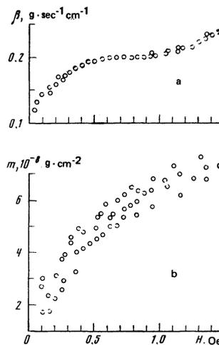
FIG. 5. Dependence of the effective viscosity  $\beta$  (a) and mass  $m$  (b) of a DB on the value of the magnetizing field  $H$ .
