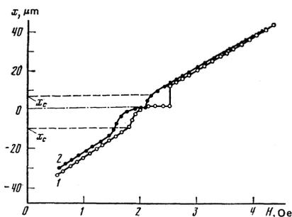
FIG. 7. Dependence of the displacement  $x$  of a DB in the elastic field of the dislocation shown in Fig. 6, from bottom to top (Curve 1) and in the opposite direction (Curve 2), on the value of the external static magnetic field. The position of the dislocation corresponds to  $x = 0$ .
