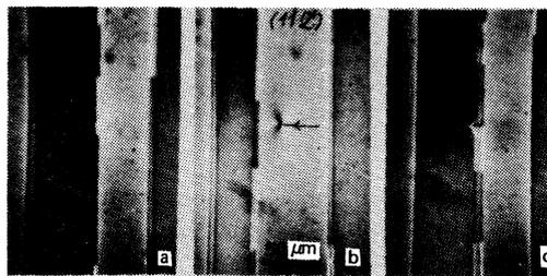
FIG. 9. Effect of the interaction of a single DB with a dislocation upon the behavior of other boundaries in the crystal, oscillating under the action of a pulsed field. The dislocation is marked by an arrow.
