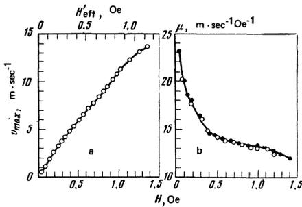
FIG. 4. Dependence of the maximum velocity (a) and of the mobility (b) of a DB on the value of the external magnetic field ( $H$ ) and of the effective magnetic field ( $H'_{eff}$ ):  $\circ$ ,  $\mu = v_{max}/H'_{eff}$ ;  $\bullet$ ,  $\mu = 2M/\beta$ .
