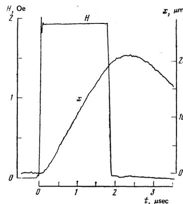
FIG. 3. Pulse of the magnetic field  $H$  and DB displacement  $x$  caused by it, recorded with an  $xy$  recorder.
