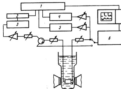
FIG. 2. Block diagram of spectrometer: 1) pulse supply unit, 2) modulator, 3)  $\omega_{ph}$  generator, 4)  $\omega_n$  generator, 5)  $2\omega_n$  generator, and 6) receiver.
