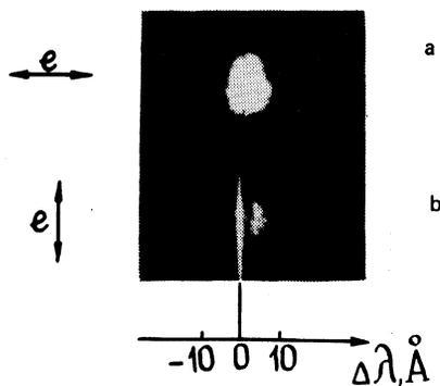
FIG. 5. Spectrograms of backscattered radiation at the fundamental frequency for two polarizations (relative to the polarization of the incident laser radiation): a) perpendicular; b) parallel.
