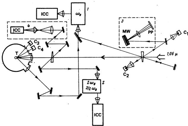
FIG. 2. Experimental setup for normal incidence of laser radiation on a target: T is a target,  $C_{1-4}$  are calorimeters; 1) SFD-1 monochromator; 2) MDR-3 monochromator; 3), 4) systems for the determination of the distribution of the laser radiation intensity on a target; PP is a photographic plate; MW is a mirror wedge; ICC is an image-converter camera.
