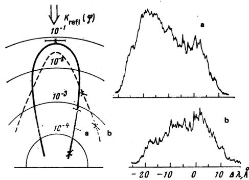
FIG. 3. Angular distributions and microphotograms of back-scattered radiation.
