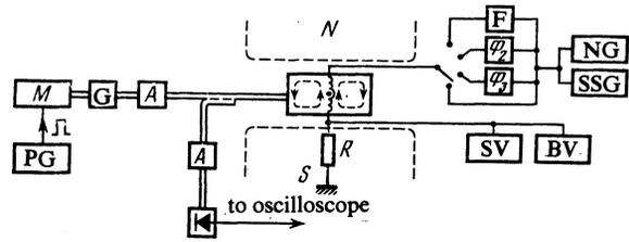
FIG. 1. Block diagram of the experimental setup. M = magnetron, PG = pulse generator, G = gate, A = attenuator, F = low-frequency filter, NG = noise generator, SSG = standard signal generator, SV = selective voltmeter, BV = broadband voltmeter.
