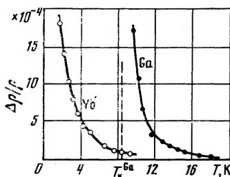
FIG. 1. Change in the magnetoresistance vs the temperature in a magnetic field of 1.6 T. The field is directed normal to the plane of the film. The thickness of the Yb and Ga films is  $\sim 10 \text{ nm}$ .
