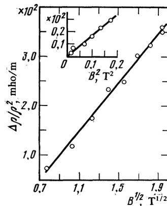
FIG. 4. Behavior of  $\Delta\rho/\rho^2$  in the field interval  $\sim 0.6$ – $3.7$  T for a Yb film 45 nm thick at 4.2 K. The inset shows the  $B^2$  dependence of  $\Delta\rho/\rho^2$  for the same film in the low-field region.
