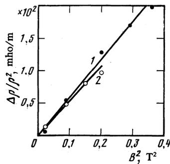
FIG. 2. 1—Dependence of  $\Delta\rho/\rho^2$  on  $B^2$  for an amorphous Bi film  $\sim 25 \text{ nm}$  thick at 7.8 K; 2—for an amorphous V film 40 nm thick at 4.2 K (weak-field region).
