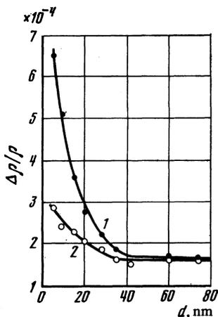
FIG. 5. Dependence of the magnetoresistance on the thickness of amorphous Yb films in a field of 1.6 T at 4.2 K. 1, 2—The magnetic field is respectively normal and parallel to the plane of the film.
