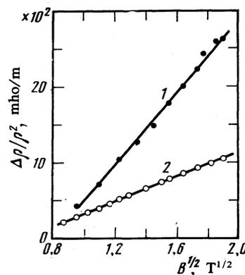
FIG. 3. Behavior of  $\Delta\rho/\rho^2$  in the field interval  $\sim 0.8\text{--}3.6 \text{ T}$  for films of Bi (1) and V (2). The samples and the experimental conditions are described in the caption of Fig. 2.
