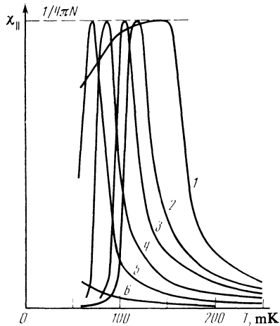
FIG. 5. Temperature dependence of the magnetic susceptibility of the solid solution \text{Ni}_x\text{Zn}_{1-x}\text{SiF}_6 \cdot 6\text{H}_2\text{O} near the ordering temperature for different concentrations of the \text{Ni}^{2+} ions: 1— x = 1 ; 2—0.72; 3—0.6; 4—0.5; 5—0.4; 6—0.18.
