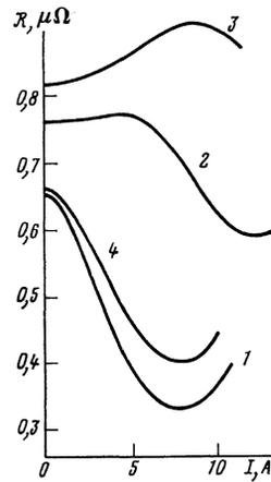
FIG. 6. Influence of an external magnetic field  $H$  on the differential resistance of tungsten plate W1 at  $T = 4.2$  K. 1)  $H = 0$ ; 2, 3)  $H = H_x = 60$  Oe and 120 Oe, respectively; 4)  $H = H_y = 100$  Oe.
