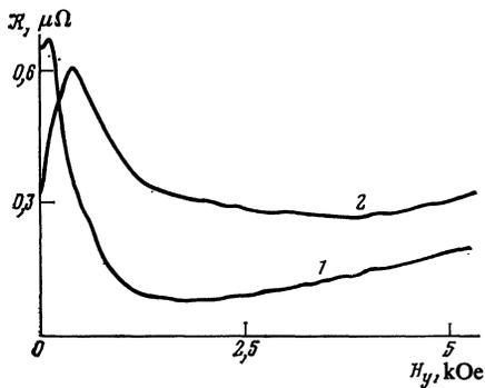
FIG. 1. Differential resistance of tungsten plate W1 in a longitudinal magnetic field,  $T = 4.2$  K. Curves 1 and 2 correspond to  $\mathcal{R}(I = 0) \approx R_0$  and  $\mathcal{R}(I = 7.5$  A), respectively.
