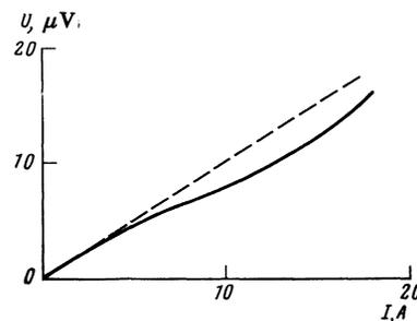
FIG. 3. Voltage-current characteristic of cadmium plate Cd1,  $T = 1.5$  K. The dashed line shows the dependence  $U = R_0 I$ .
