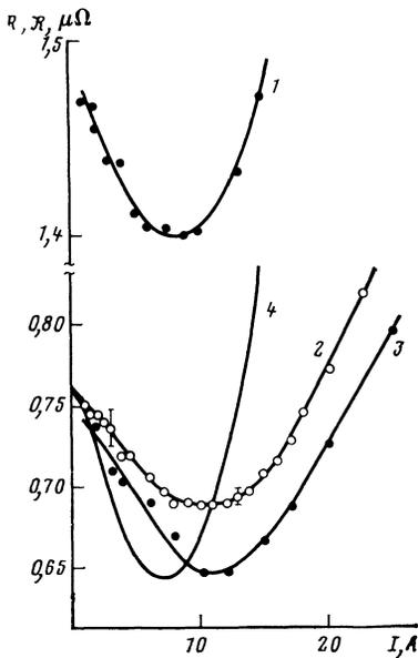
FIG. 4. Resistance (curves 1-3) and differential resistance (curve 4) of tungsten plates as a function of the current. 1) W3 plate,  $T = 1.5$  K; 2, 3) W4 plate,  $T = 4.2$  and  $1.5$  K; 4) W4 plate,  $T = 4.2$  K.
