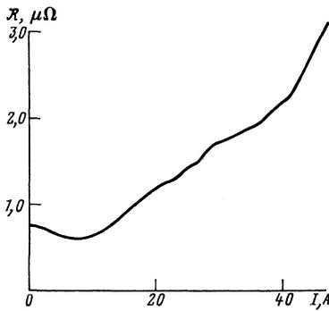
FIG. 5. Differential resistance of plate W4 for a wide range of currents,  $T = 2.2$  K.
