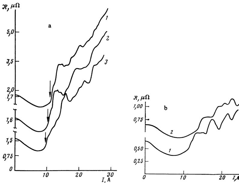
FIG. 7. Oscillations of the differential resistance as a function of the current. a) Plate W2,  $H = 0.1$ )  $T = 4.2$  K; 2)  $T = 3.4$  K; 3)  $T = 1.5$  K; b) Plate W1,  $T = 4.2$  K; 1)  $H = 0$ ; 2)  $H = H_x = 20$  Oe.
