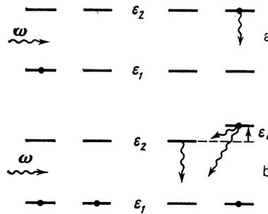
FIG. 1. a) Initial and final states of an electron in intercenter phototransition to an empty center, b) intercenter phototransition to an occupied center; the wave lines represent the recombination channels.
