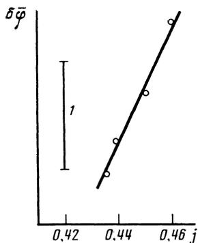
FIG. 8. Current-voltage characteristic of a superconducting domain with a PSC;  $\delta\bar{\varphi} = \delta\bar{\varphi}(j)$ .
