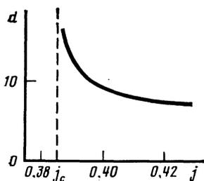
FIG. 3. Dependence  $d(j)$  of the period of the PSC lattice on current in a conductor.
