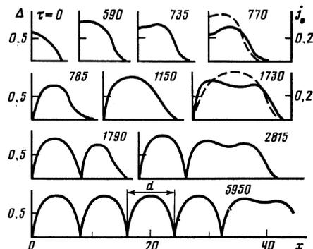
FIG. 2. Formation of a PSC lattice in a normal conductor for  $j > j_c$ .
