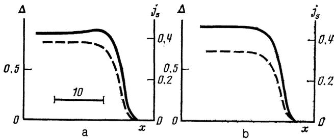
FIG. 5. Wave of transformation to the superconducting state: (a)  $j = 0.38$ , (b)  $j = 0.34$ .
