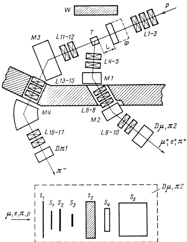
FIG. 1. Experimental setup:  $M_1$ – $M_4$ ) turning magnets;  $L_1$ )– $L_{17}$ ) quadrupole lenses;  $T$ ) meson-producing target;  $W$ )—protecting wall;  $D\pi_1$  and  $D\mu, \pi_2$ ) muon and pion detectors;  $t_1, t_2$ ) copper filters;  $S_1$ – $S_5$ ) scintillation counters.
