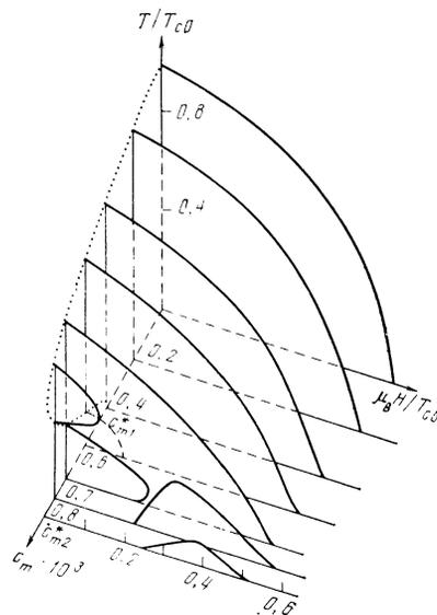
FIG. 2.  $(T, H)$  diagrams of the superconductor for various values of the concentration of magnetic impurities ( $\xi_0/a = 50$ ).
