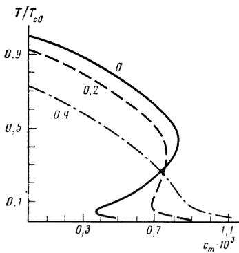
FIG. 1. Superconducting transition temperature as a function of the concentration of magnetic impurities at various values of the external magnetic field ( $\xi_0/a = 50$ ).
