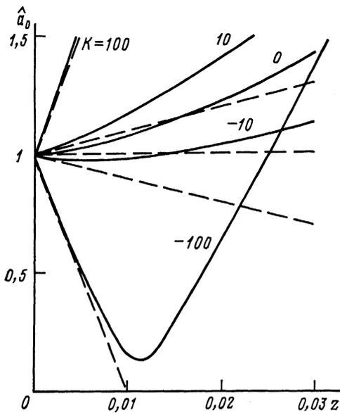
FIG. 3. Dependence of the dimensionless radius of the beam  $\hat{a}_0 = a_0/a$  on the coordinate  $z$  at  $\Pi = 10$  and for various curvatures of the wavefront  $K$ . The medium is defocusing:  $\delta > 0$ . The dashed lines are the corresponding dependences in the absence of self-action ( $\Pi \rightarrow 0$ ).
