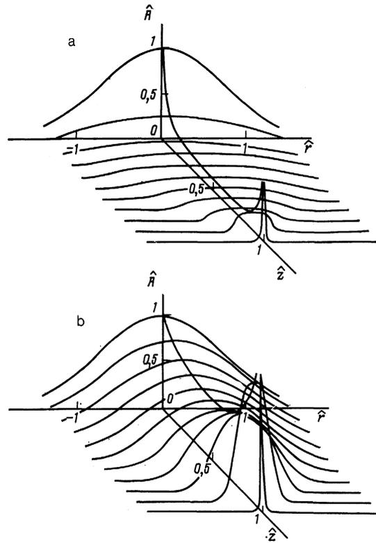
FIG. 1. Distribution of wave amplitude in self-focusing ( $\hat{A} = A/p_0$ ,  $\hat{z} = z/z_f$ ,  $r = r/a$ ): a— $\Pi = 0.1$ ,  $z_f = 203$ ; b— $\Pi = 1$ ,  $z_f = 2.36$ .
