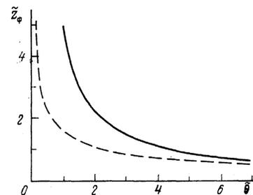
FIG. 5. Coordinate of the point of "collapse"  $\tilde{z}_c$  as a function of the time  $\tilde{\theta}$ . The dashed curve is the corresponding  $\tilde{z}_c^*(\tilde{\theta})$  dependence from the solution of the approximate self-similar equation.
