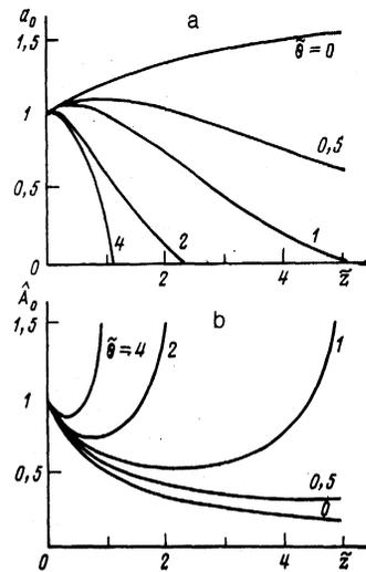
FIG. 4. Dependence of the beam characteristics on the distance  $z$  at successive instants of time  $\tilde{\theta}$  for the case  $\tilde{K} = 0$ ,  $\delta < 0$ ;  $a - \hat{a}_0 = a_0/a$  is the dimensionless beam radius.  $b - \hat{A}_0 = A_0/p_0$  is the dimensionless amplitude of the wave on the axis.
