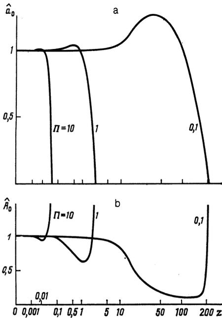
FIG. 2. Dependence of the beam characteristics on the distance  $z$  for various wave amplitudes  $\Pi$ :  $a-\hat{a}_0 = a_0/a$  is the dimensionless radius of the beam;  $b-A = A_0/p_0$  is the dimensionless amplitude of the wave on the axis.
