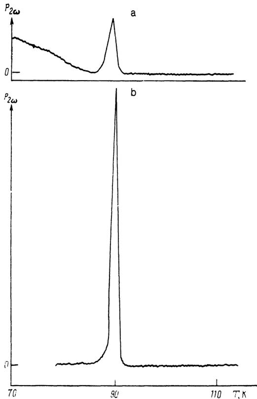
FIG. 1. Dependences of the second-harmonic power  $P_{2\omega}$  on the temperature for ceramic (a) and single-crystal (b) samples of YBaCuO. Frequency  $\omega/2\pi = 9.4$  GHz, external magnetic field  $H = 20$  Oe, the maximum amplitude of the alternating magnetic field  $H_{\omega} \parallel H$  on the sample surface is  $H_{\omega} = 18$  Oe (a) and 15 Oe (b).
