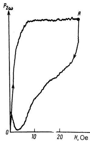
FIG. 3.  $P_{2\omega}(H)$  dependence in single-crystal YBaCuO for  $T \approx T_c$ ;  $H_{\omega} = 10$  Oe and  $\omega/2\pi = 9.4$  GHz. The direction of the current variation was reversed at the point A.
