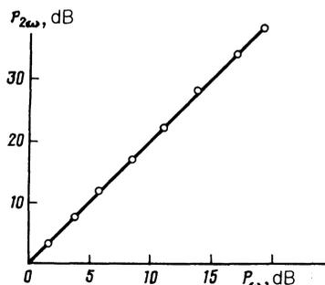
FIG. 2.  $P_{2\omega}(P_{\omega})$  dependence in single crystal YBaCuO at  $T \approx T_c$ ;  $H \parallel H_{\omega}$ ,  $H = 15$  Oe and  $\omega/2\pi = 9.4$  GHz.
