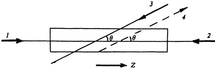
FIG. 2. Diagram of wavefront conjugation for degenerate four-wave interaction.
