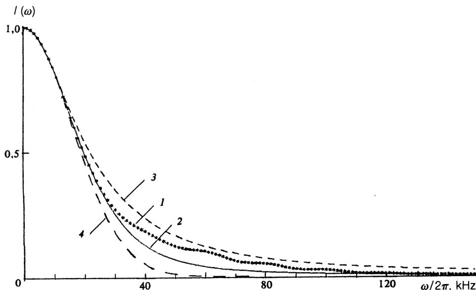
FIG. 2. NMR line profile for a suspension with PM-1 powder: 1—experiment, 2—Fourier transform of the expression (9), 3—Lorentzian, 4—Gaussian.
