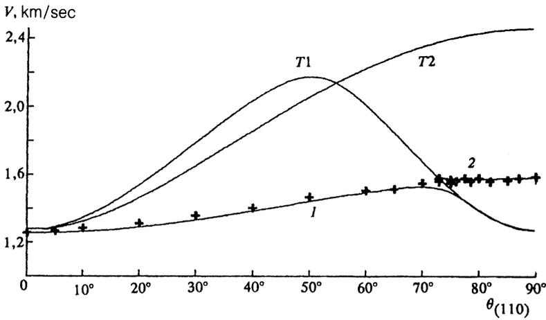
FIG. 2. Velocities of GSW, pseudosurface,  $T_1$ , and  $T_2$  acoustic waves for the (110) plane in PbTe as a function of the angle  $\theta_{(110)}$ . The crosses are the experimental values of the GSW and pseudosurface mode velocities; the solid lines are the theoretical curves for GSW (1), pseudosurface (2),  $T_1$ , and  $T_2$ . The values of the material parameters for the curves presented were taken from Ref. 19.
