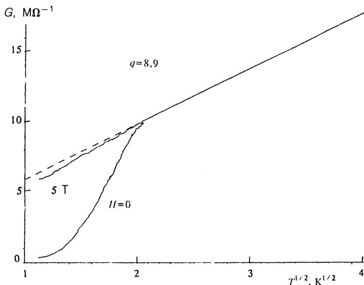
FIG. 5. Reconstruction, by a magnetic field, or "normal" conductivity of a highly resistive state of a sample. Dashed—continuation of the  $G(T^{1/2})$  straight plot of the experimental data at  $T > T_c$ . The data in Figs. 5–8 were obtained in the same sample state,  $q=8, 9$ , as in Figs. 3 and 4, but at shorter distances between the contacts.
