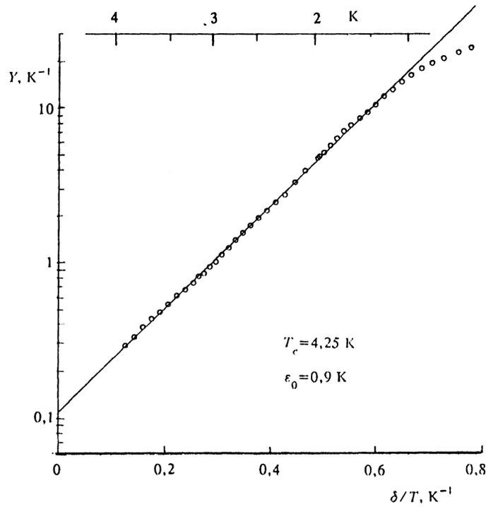
FIG. 7. Reduction of the experimental temperature dependence of the resistance, to determine the value of the superconducting gap from the  $R(T)$  curve with  $\partial R/\partial T < 0$  (see the text).
