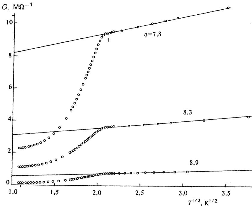
FIG. 3. Temperature dependence of the conductivity of three high-resistance states of a sample.
