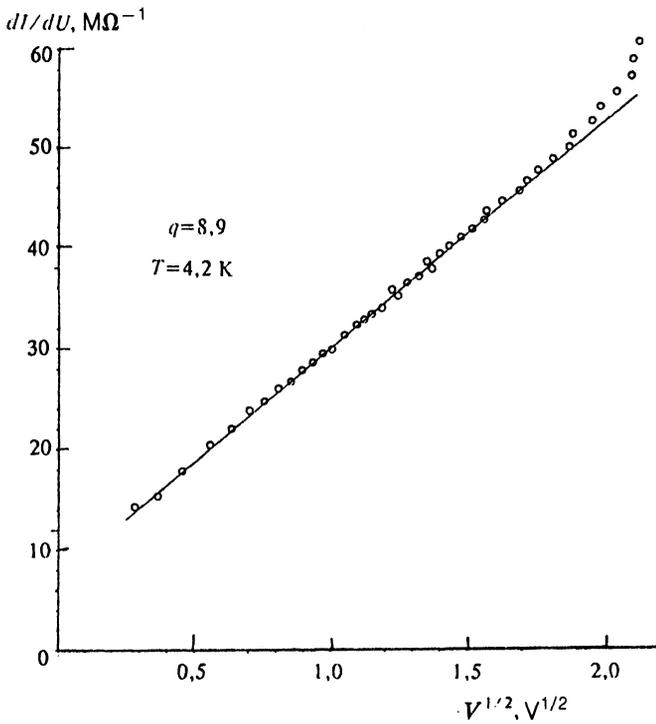
FIG. 8. Square-root dependence of the differential conductivity of a highly resistive state of a sample on the voltage applied to the sample.
