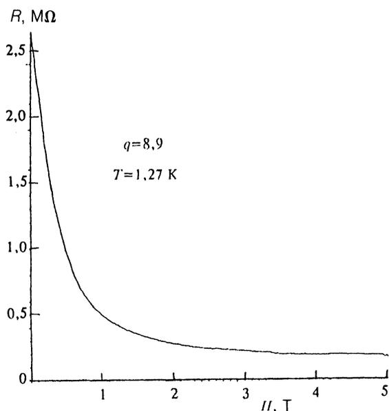
FIG. 6. Giant negative magnetoresistance at  $T=1.27$  K.
