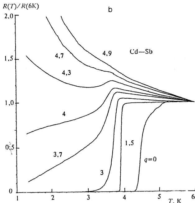
FIG. 2. Evolution of superconducting response in the alloys Ga-Sb (a) and Cd-Sb (b) in various states of the samples. All the  $R(T)$  curves are normalized to the resistance at  $T=6$  K. The parameter  $q$  is defined by Eq. (3).
