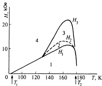
FIG. 2. Phase  $H-T$  diagram for Dy for  $H \parallel a$ . Phases: 1) "simple helix"; 2) intermediate (domain) phase; 3) fan; 4) collinear phase. Curves  $H_1, H_2, H_3$  correspond to the phase transitions.
