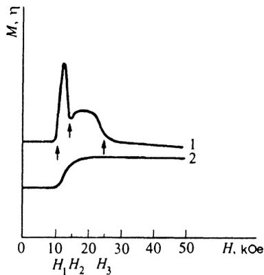
FIG. 1. Experimental dependences of the EMAT efficiency  $\eta$  (curve 1) and of the magnetization  $M$  (curve 2) on the magnetic field in dysprosium at  $T=173$  K (Ref. 3). The magnetic fields marked by arrows correspond to the phase transitions "simple helix"-intermediate (domain) phase ( $H_1$ ); intermediate phase-fan ( $H_2$ ); and fan-collinear phase ( $H_3$ ).
