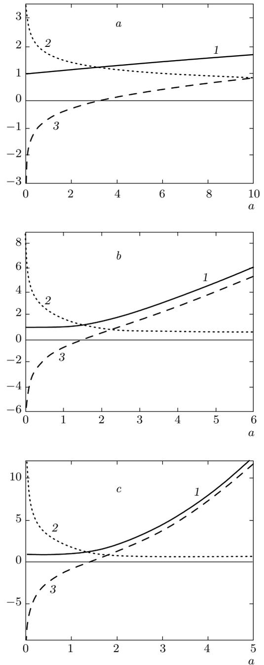
**Fig. 1.** Energy  $E$  (1), heat  $Q$  (2), and work  $W$  (3), Eqs. (21)–(24), for different values of the parameter  $w = 0$  (a),  $-0.6$  (b), and  $-1$  (c) in the equation of state  $p = w\rho$ . The first principle of thermodynamics  $E = Q + W$  is always satisfied
