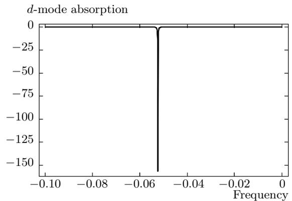
**Fig. 4.** Total absorption  $1 - |T(d, L)|^2 - |R(d, L)|^2$  versus the frequency for an amplifying defect layer and nonabsorbing CLC layers at  $g = -0.0065957$  for  $d/p = 0.25$
