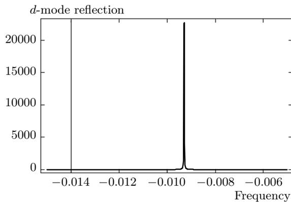
**Fig. 6.** Reflection  $|R(d, L)|^2$  versus the frequency for an amplifying defect layer and nonabsorbing CLC layers at  $g = -0.04978$  for  $d/p = 0.1$
