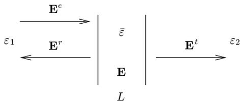
Fig. 10. Schematic of the CLC edge mode structure with dielectric jumps at the interfaces
