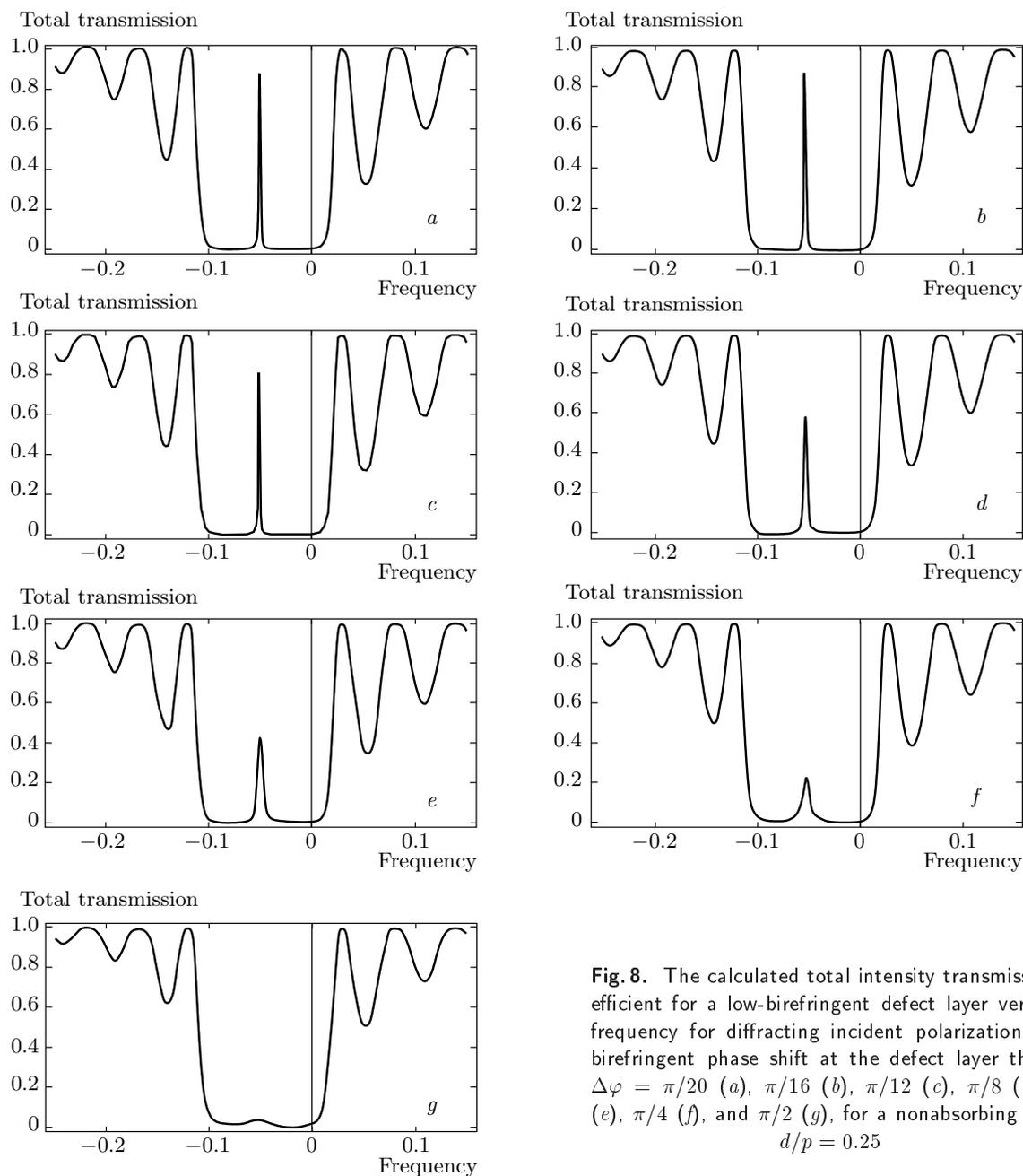
**Fig. 8.** The calculated total intensity transmission coefficient for a low-birefringent defect layer versus the frequency for diffracting incident polarization at the birefringent phase shift at the defect layer thickness  $\Delta\varphi = \pi/20$  (a),  $\pi/16$  (b),  $\pi/12$  (c),  $\pi/8$  (d),  $\pi/6$  (e),  $\pi/4$  (f), and  $\pi/2$  (g), for a nonabsorbing CLC at  $d/p = 0.25$
