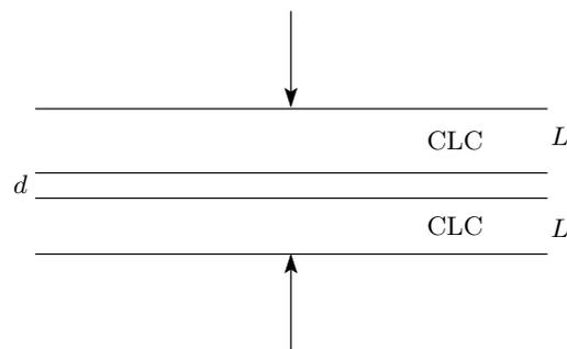
**Fig. 1.** Schematic of the CLC defect mode structure with an isotropic active defect layer of thickness  $d$
