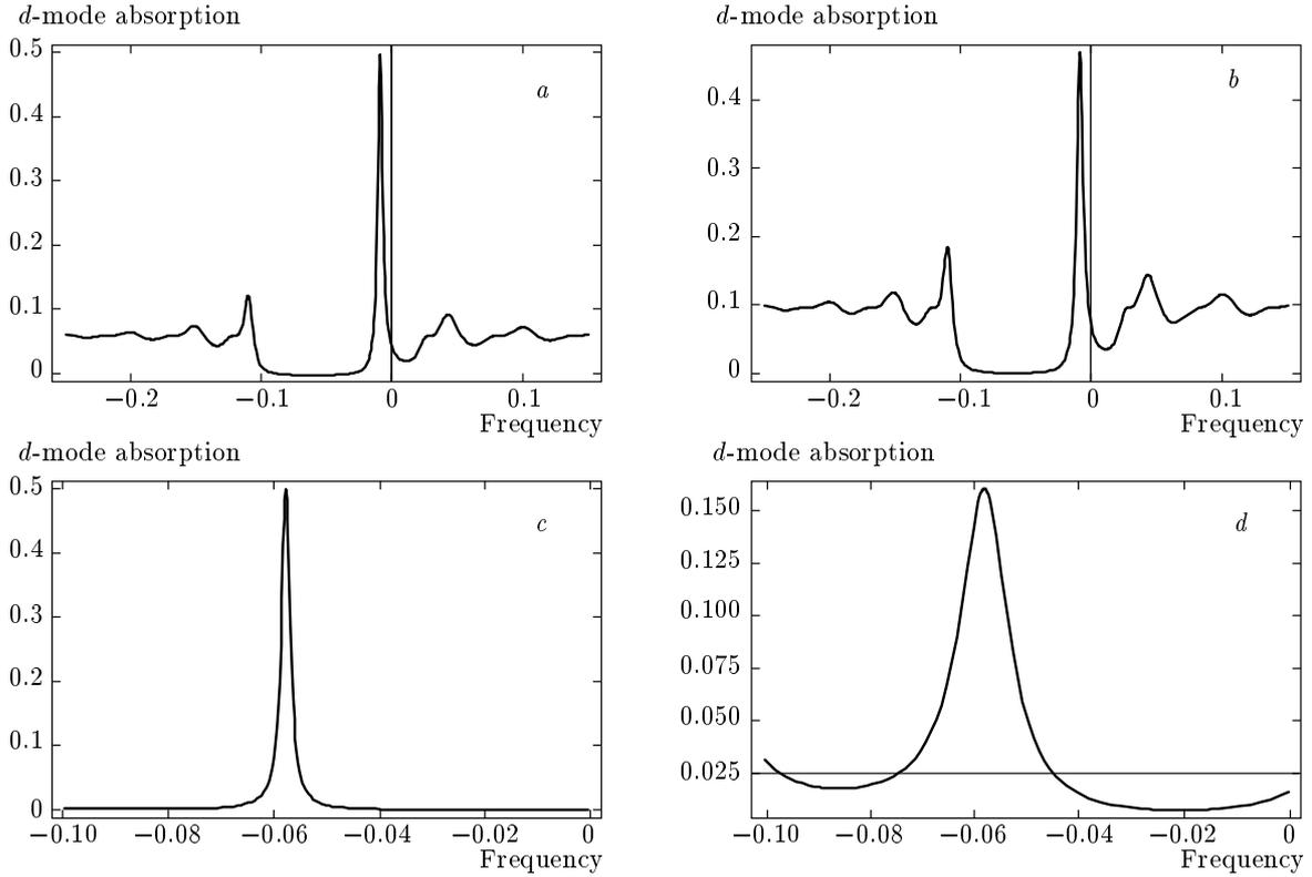
**Fig. 3.** Total absorption  $1 - |T(d, L)|^2 - |R(d, L)|^2$  versus the frequency for an absorbing defect layer and nonabsorbing CLC layers at  $g = 0.04978$  (a),  $0.08$  (b) for  $d/p = 0.1$ ; at  $g = 0.00008891$  (c),  $0.0008891$  (d) for  $d/p = 22.25$
