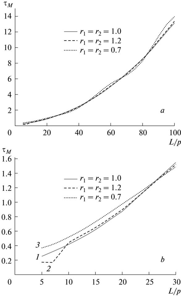
**Fig. 11.** *a)* The calculated EM lifetime versus the CLC layer thickness normalized by the CLC layer flight time  $\varepsilon_0^{1/2}L/c$  for several values of the dielectric jump at the CLC layer surface, *b)* magnified part of Fig. 11*a*
