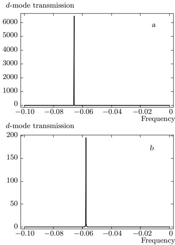
**Fig. 5.** Transmission  $|T(d, L)|^2$  versus the frequency for an amplifying defect layer and nonabsorbing CLC layers at  $g = -0.001000$  for  $d/p = 2.25$  (a) and  $g = -0.00008891$  for  $d/p = 22.25$  (b)
