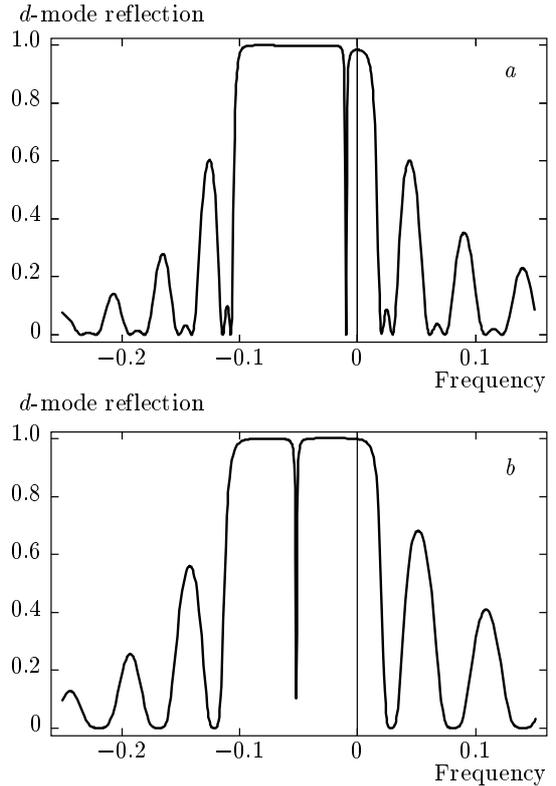
**Fig. 2.** Reflection  $|R(d, L)|^2$  versus the frequency for a nonabsorbing defect and CLC layers ( $g = 0$ ) at  $d/p = 0.1$  (a), 0.25 (b);  $l = 200$ ,  $l = L\tau = 2\pi N$ , where  $N$  is the director half-turn number at the CLC layer thickness  $L$ . Here and on figures below,  $\delta = 0.05$ , the director half-turn number at the CLC layer thickness is  $N = 33$ , frequency  $\nu = \delta[2(\omega - \omega_B)/\delta\omega_B - 1]$
